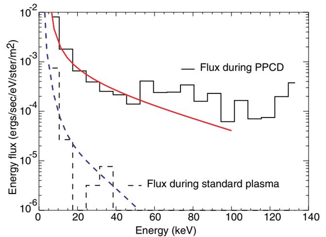
FIG. 2 (color online). Measured HXR flux for standard plasma (dashed histogram) is best fit (dashed curve) using a diffusion coefficient proportional to the parallel electron velocity ( $\alpha = 1$ ). Measured HXR flux in improved confinement plasma (solid histogram) is best fit (solid curve) using diffusion coefficient which is velocity independent ( $\alpha = 0$ ).
