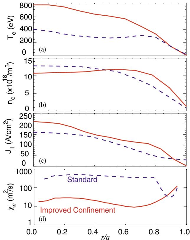
FIG. 1 (color online). Radial profiles of plasma parameters during standard discharges (dashed lines) and PPCD (solid lines), (a) the electron temperature, (b) the electron density, (c) the parallel current density and (d) the electron heat diffusivity.
