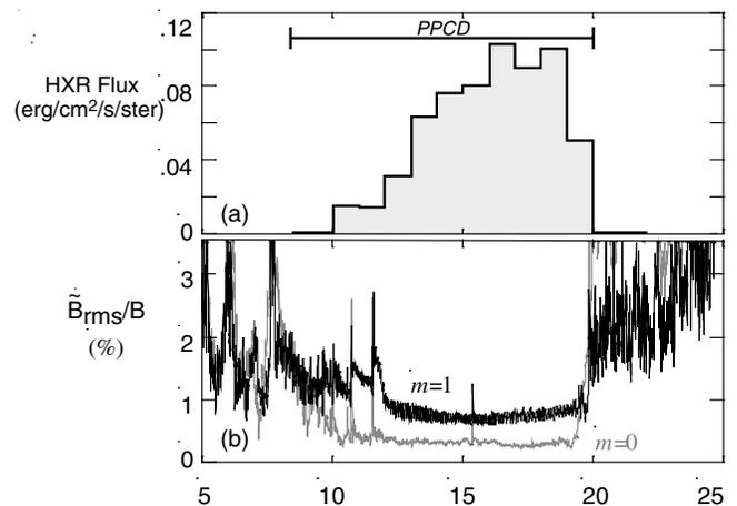
FIG. 3. The integrated HXR flux for energy beyond 20 keV (a) and the rms fluctuation amplitude as a percentage of the equilibrium field (b) versus time for a 400 kA improved confinement PPCD discharge. Modeling shows that this flux corresponds to a runaway electron population of  $\sim 1$ –2%.
