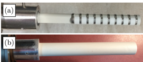
FIG. 1. A multi-channel linear capacitive probe without BN particle shield (a) and with BN particle shield (b).
