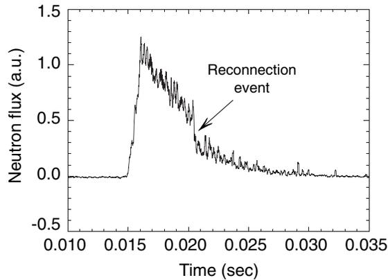
FIG. 4. Waveform of neutron flux with a reconnection event at  $t = 0.02$  s. During the  $\sim 200 \mu\text{s}$  duration of the event, the neutron flux drops by a factor of 2. After the event the slow decay is resumed.
