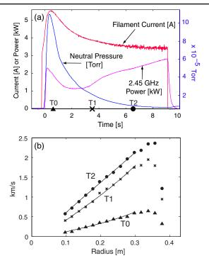
FIG. 2 (color online). (a) Typical plasma discharge: plasma density decreases and electron temperature increases as the puff of neutral gas is pumped out. (b) Velocity profiles in argon at times labeled in (a) for two cathodes biased to 400 V. Rotation increases at low density and high ionization fraction. Solid lines represent a model incorporating unmagnetized Braginskii viscosity and neutral drag (due to charge exchange), using parameters from Table I.
