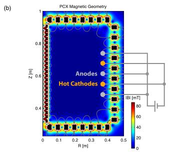
FIG. 1 (color online). The Plasma Couette Experiment (PCX). (a) Experimental setup showing the vacuum vessel, internal structure of the ring cusps, and diagnostic layout. (b) Poloidal cross section showing magnetic geometry and stirring electrodes; black rectangles are permanent magnets, white lines show resonance surfaces for electron-cyclotron heating (|B| = 87 mT), gray lines show cusp field lines.
